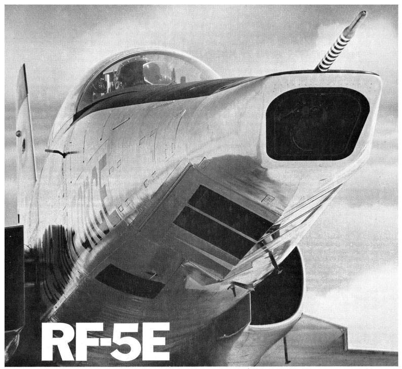
New multi-role reconnaissance version of Northrop's F-5E Tiger II. Modified nose section contains 26 cubic feet of space—nearly nine times more than RF-5A—for broad range of sensors currently in use by U.S. Air Force.
