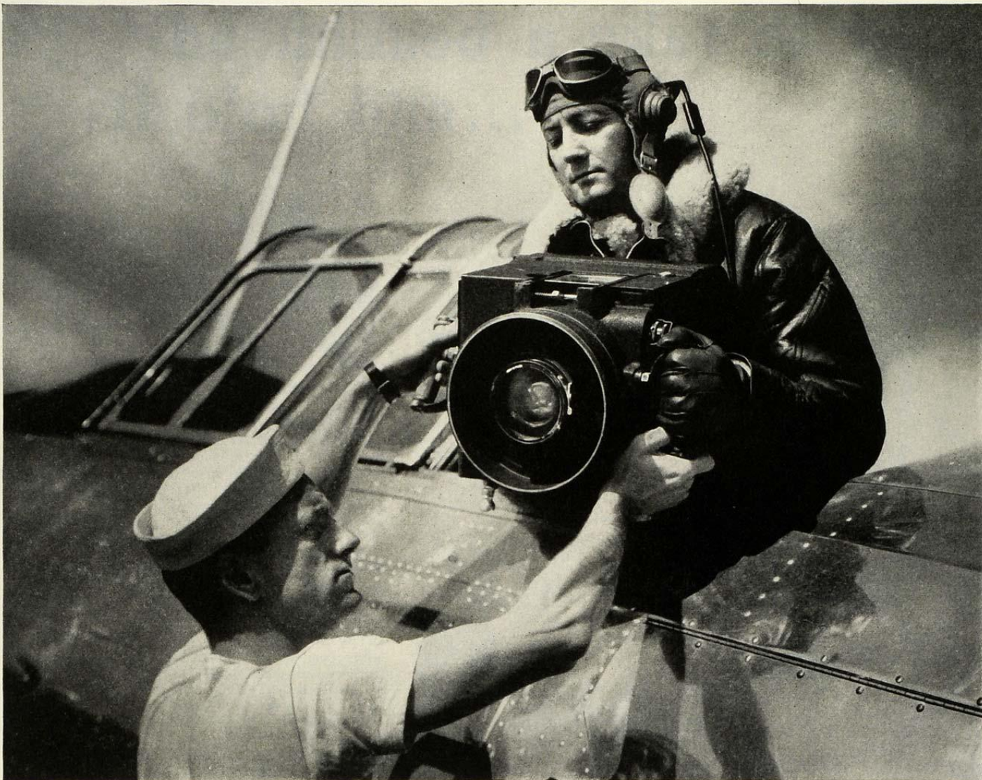
B&L Altimar f:4 lens in Fairchild (F-56) Aerial Camera.
